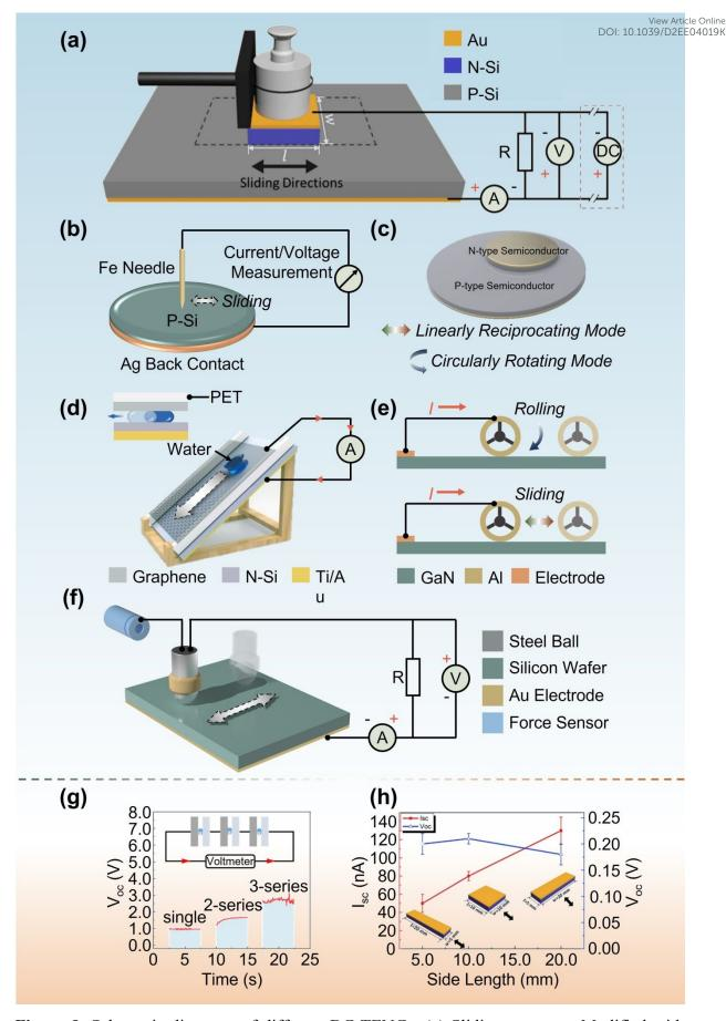
**Figure 9.** Schematic diagrams of different DC-TENGs. (a) Sliding structure. Modified with permission from ref.<sup>11</sup> Copyright 2019 Elsevier Ltd. (b) Needle tip structure. Modified with
