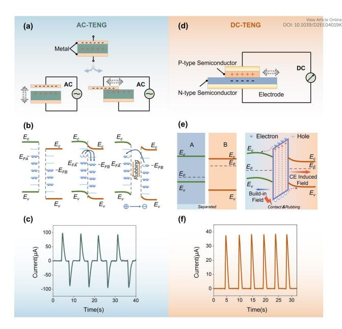
**Figure 2.** Comparison between the AC-TENG and DC-TENG based on the tribovoltaic effect. (a) Vertical contact-separation mode and lateral-sliding mode of the AC-TENG. (b) Working mechanism of the AC-TENG. (c) Basic electrical characteristics of the AC-TENG. (d) Device structure of the DC-TENG based on the tribovoltaic effect. (e) Working mechanism of the DC-TENG based on the tribovoltaic effect. (f) Basic electrical characteristics of the DC-TENG based on the tribovoltaic effect.
